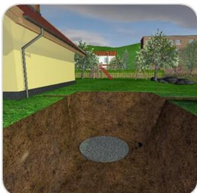
In case of plastic WWTP, a compacted gravel bed must be placed in the trench bottom. Thickness of the layer is 100 mm in the compacted state.
