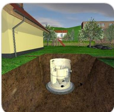
Place the waste water treatment plant on the ferro-concrete baseplate. The height of waste water treatment plant's tank is specified in the documents to specific WWTP type. If the installation depth exceeds the WWTP tank height a plastic extension piece must be extra ordered - its maximum height is given in the documents to specific WWTP type. The extension piece height needs to be consulted with the WWTP manufacturer.
